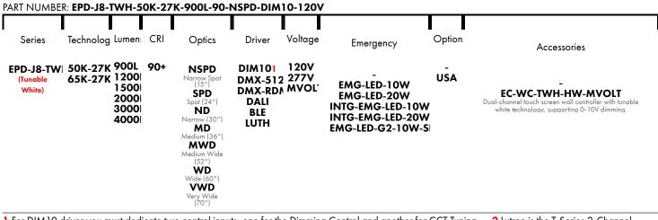
1 For DIM 10 driver you must dedicate two control inputs, one for the Dimming Control and another for CCT Tuning
